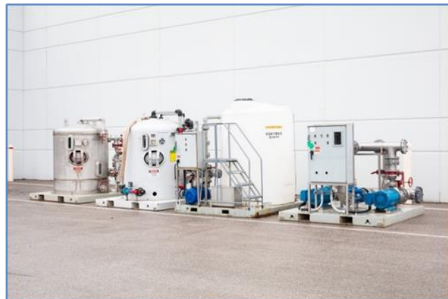
Figure 6: Veolia proprietary multi vessel water purification system with interstage testing and automation control
